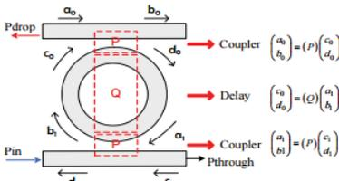
Figure 3: Coupler and delay unit of micro-ring resonator
