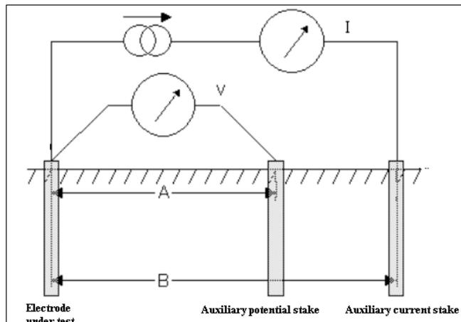
Figure 6: Schematic for the three-terminal resistance measurement.
