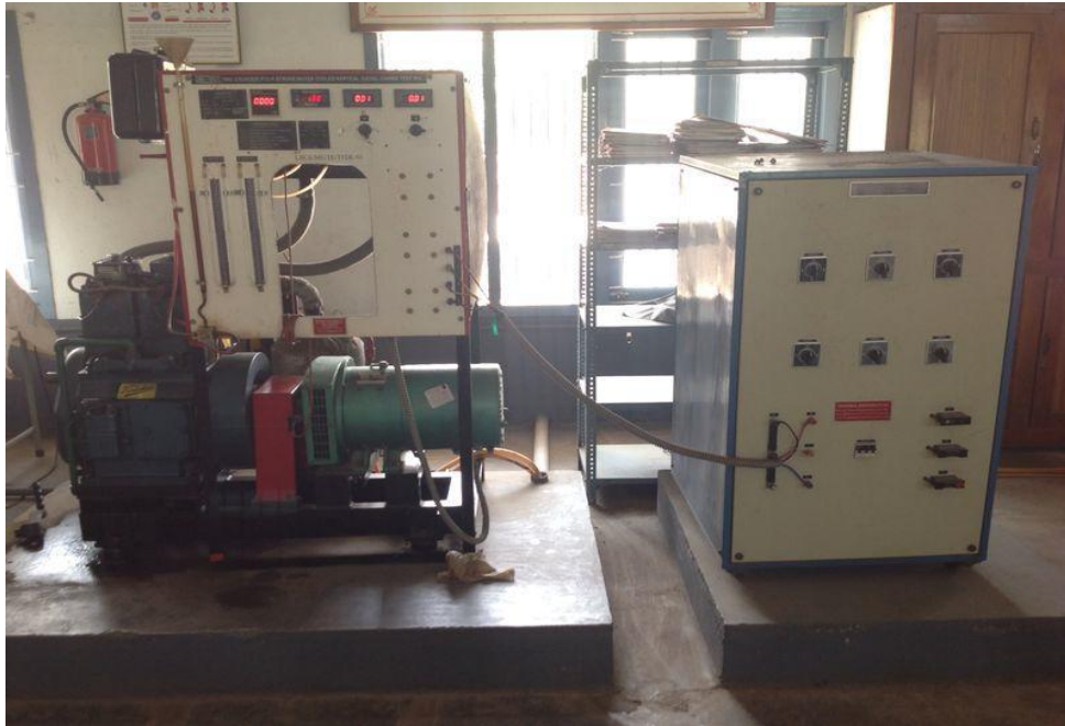
Figure 1. Four stroke twin cylinder water cooled diesel engine
