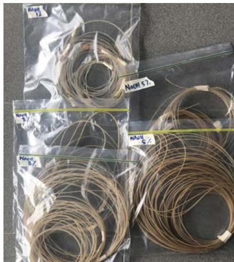
Figure 5: PALF/PLA composites filaments.
