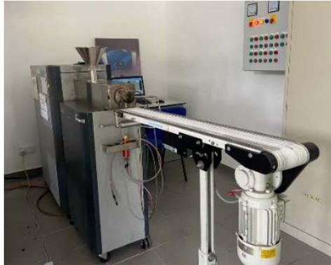
Figure 4: Single-screw extruder machine.
