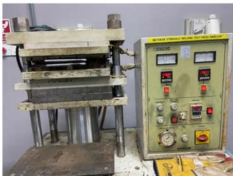
Figure 3: Hot compression machine running the composite development.
