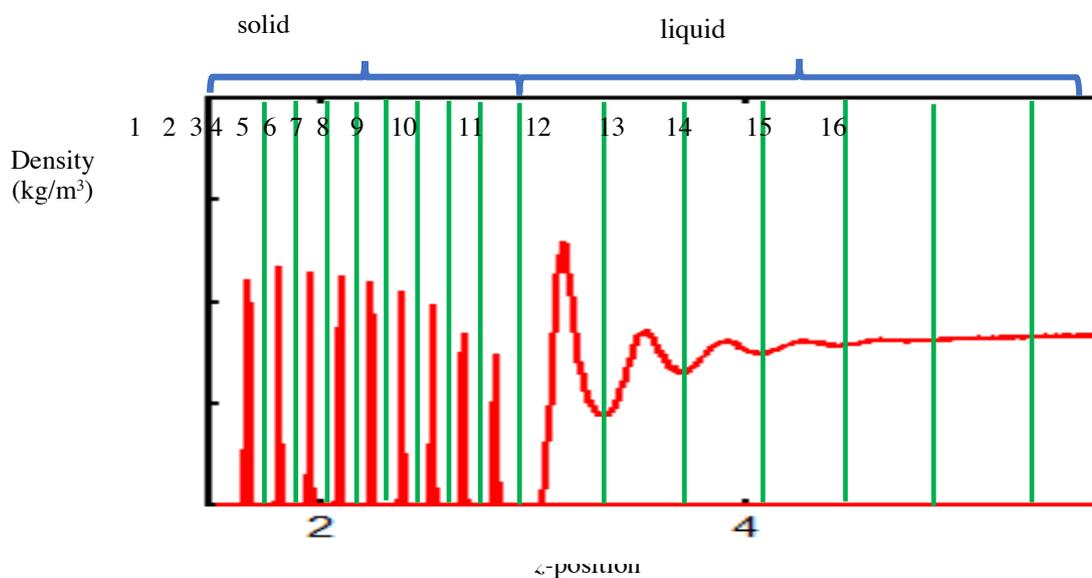
Figure 4. Slab definition for temperature distributions
