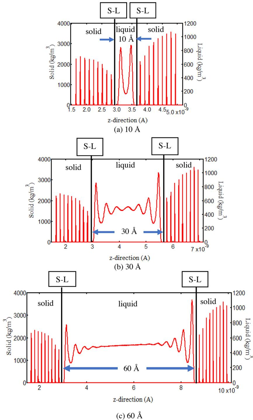
Figure 3. Density distributions for simulation model with liquid thicknesses of (a) 10 Å, (b) 30 Å, and (c) 60 Å.
