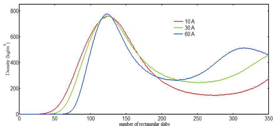
Figure 2. First adsorption layer for simulation model with liquid film thicknesses of 10 Å (red line), 30 Å (green line), and 60 Å (blue line).
