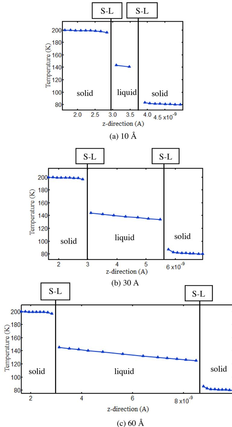
Figure 5. Temperature distribution for liquid film thicknesses for (a) 10 Å, (b) 30 Å, and (c) 60 Å.
