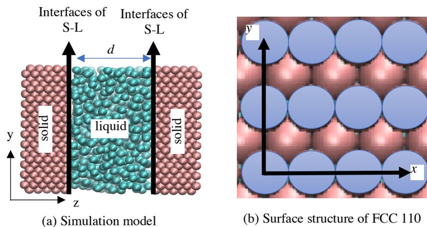
Figure 1.(a) Simulation model and (b) surface structure FCC110.
