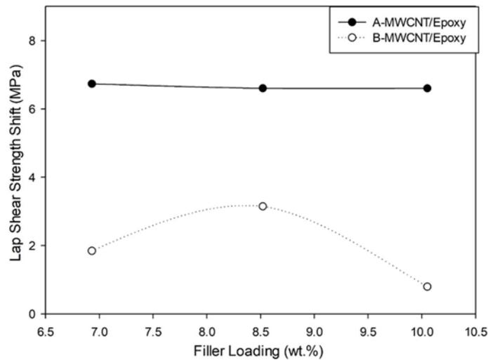
Figure 9. Shear strength shift for A-MWCNT/Epoxy and B-MWCNT/Epoxy ECAs
