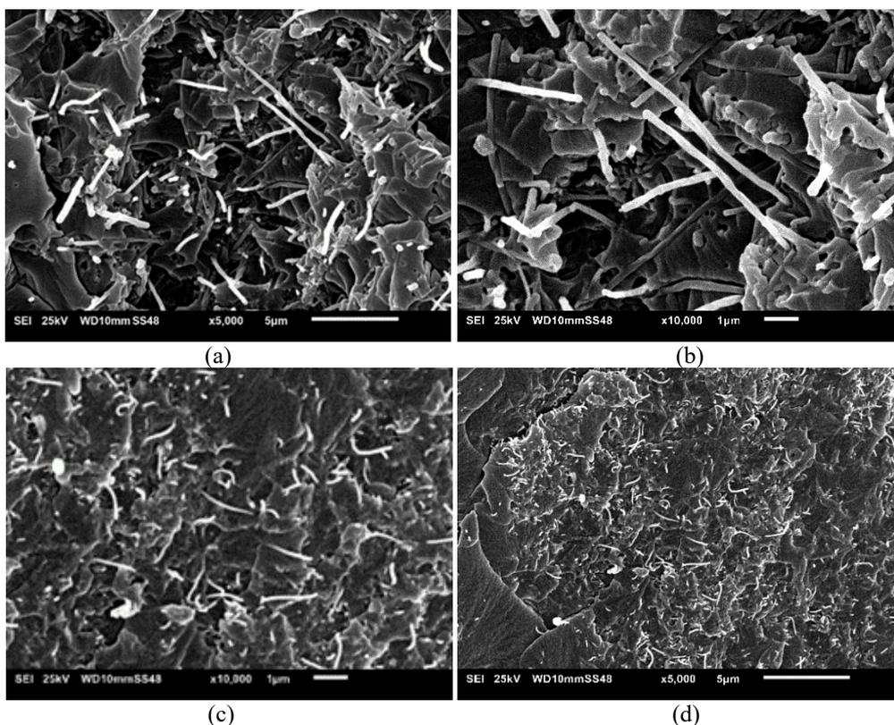
Figure 4. SEM micrographs showing the cross-sectional view of ECA with 10.05 wt.% filler loading for (a) & (b) A-MWCNT/Epoxy and (c) & (d) B-MWCNT/Epoxy, at 5000x and 10000x magnification respectively.
