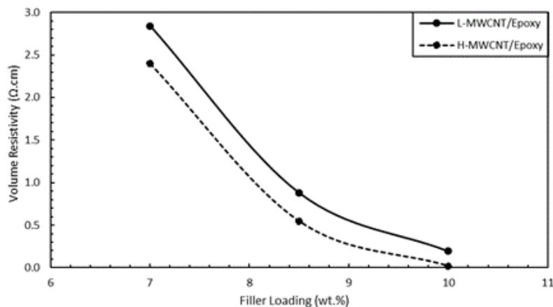
Figure 3. Volume resistivity against filler loading for L-MWCNT/Epoxy and H-MWCNT/Epoxy
