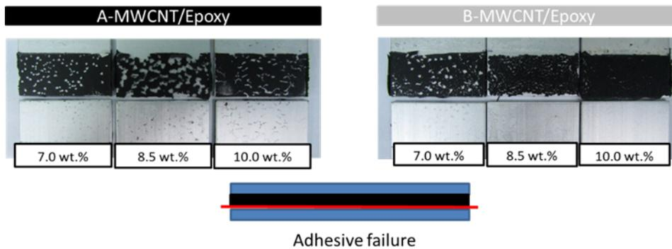
Figure 8. Surface failure for ECAs at 85 °C temperature and 85 % relative humidity
