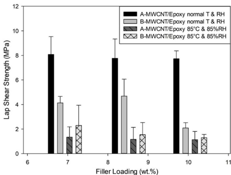
Figure 6. Shear strength of ECA at normal and elevated temperature and humidity
