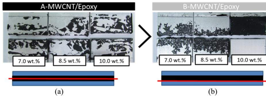
Figure 7. Surface failure of the ECA subjected to normal temperature and relative humidity, showing (a) adhesive-cohesive failure and in (b) adhesive failure
