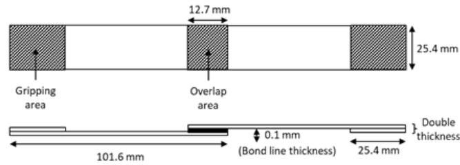
Figure 2. Sample assembly for single-lap bonded joint test
