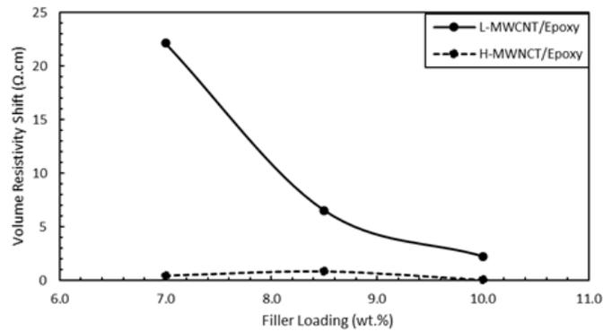
Figure 5. Volume resistivity shift after aged in 85 °C and 85 %RH for 96 hours
