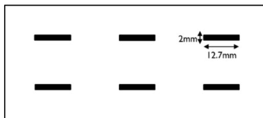
Figure 1. Schematic diagram of printed ECA arrangement
