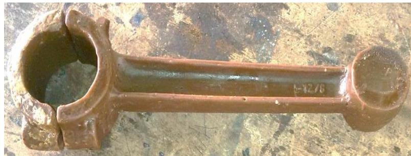
Figure 5: Pictorial view of wax pattern produced
