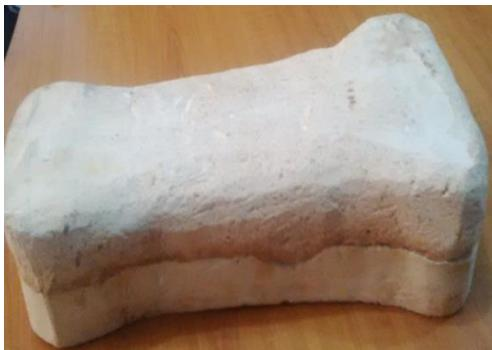
Figure 3: Pattern Mould Box for the Connecting Rod
