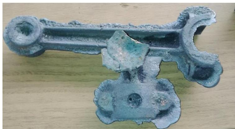
Figure 6: Connecting rod and cap produced by lost wax casting before machining
