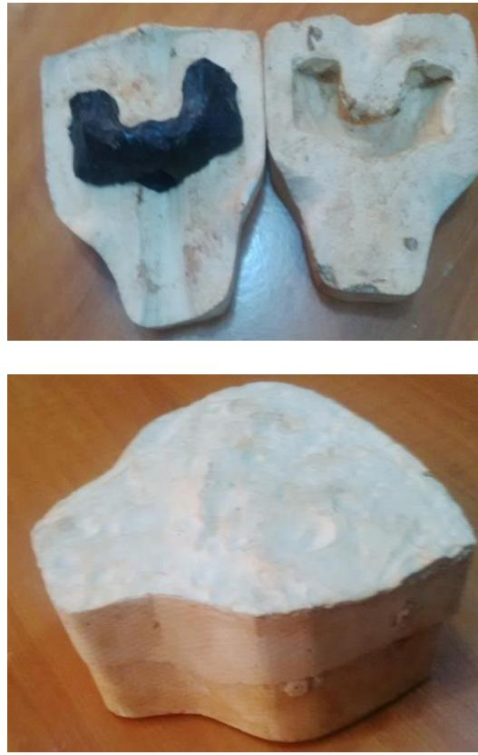
Figure. 4: Pattern Mould Box for the Connecting Rod Cap
