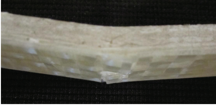
FIGURE 16 Tensile failure at mid-bottom surface
