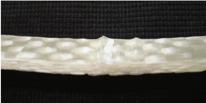
FIGURE 14 Compressive failure at mid-top surface
