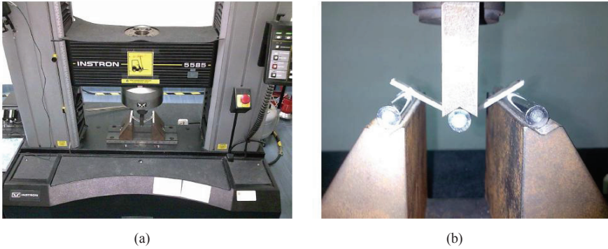
FIGURE 4 Machine and fixture (a) Instron® 5585 Universal Testing Machine, (b) Three-point fixture
