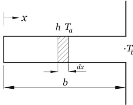
Figure 1. Schematic of the longitudinal straight fin geometry
