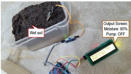
Fig. 12. LCD Output based on wet soil condition
