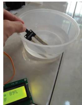
Fig. 9. Moisture sensor test for wet condition
