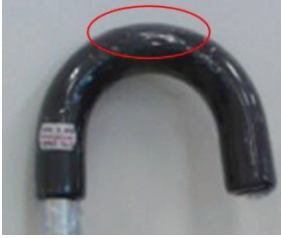
Fig. 4. Handle C. The contact point is concentrated on the top side
