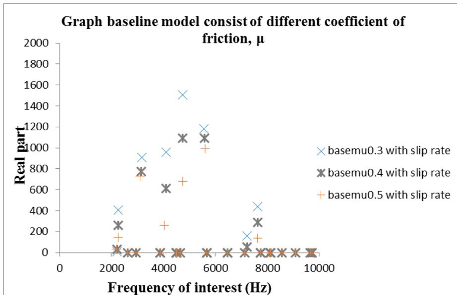
Figure 2. Relationship between frequency and brake squeal generation.
