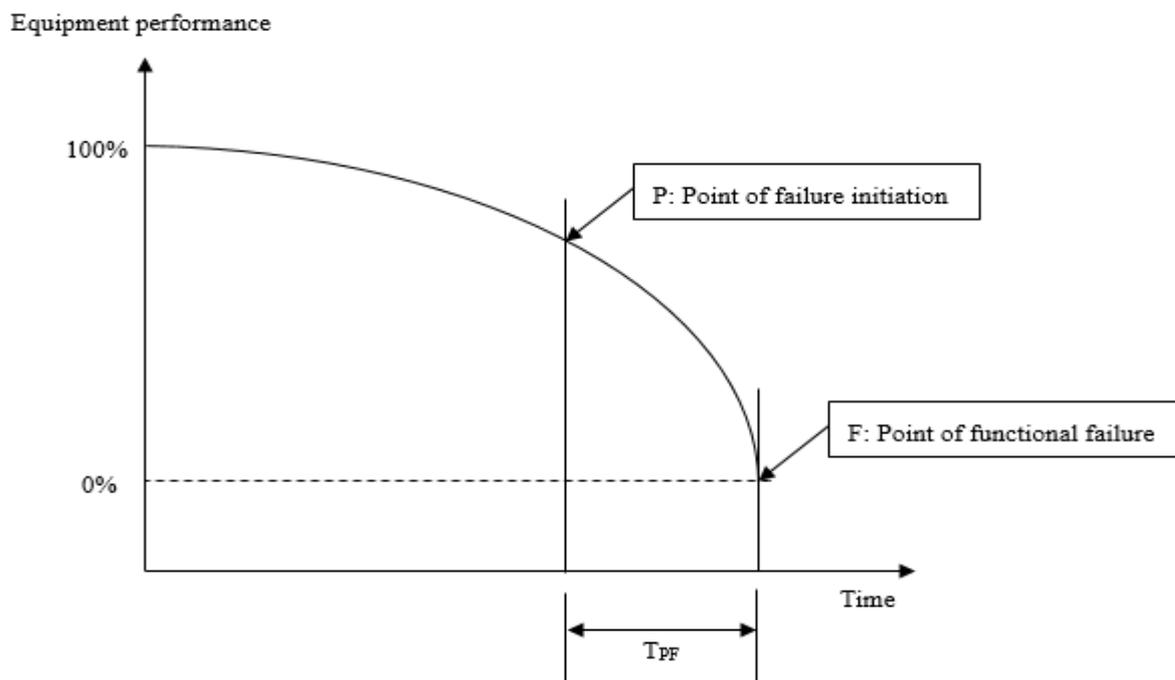
Figure 3. P-F interval (Rausand, 1998)
