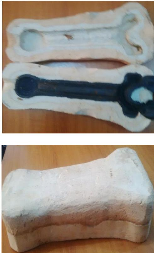
Figure 3: Pattern Mould Box for the Connecting Rod
