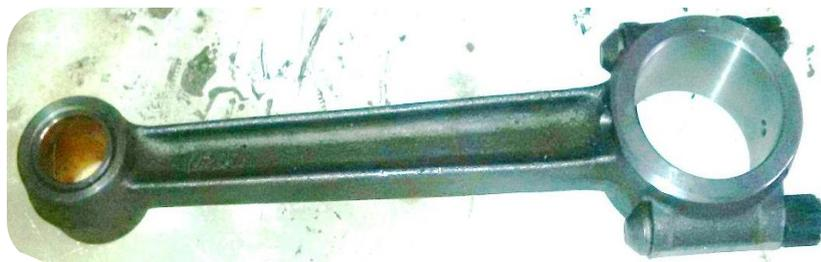
Figure 1: Sample-Connecting Rod Sourced from the 8hp Diesel Engine
