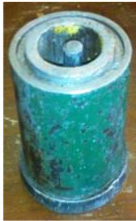
Figure 3 Metal mould used for the briquette
