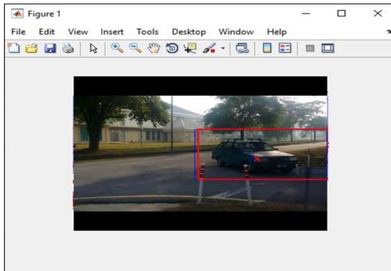
Figure 5: Detecting vehicles in shadow of tree
