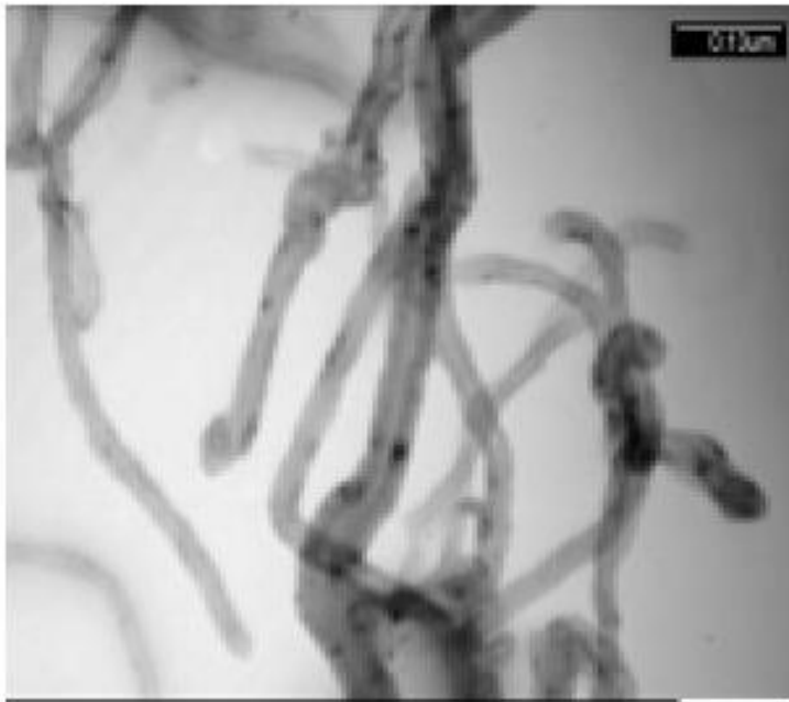
Fig.1 TEM image of purified MWNTs
