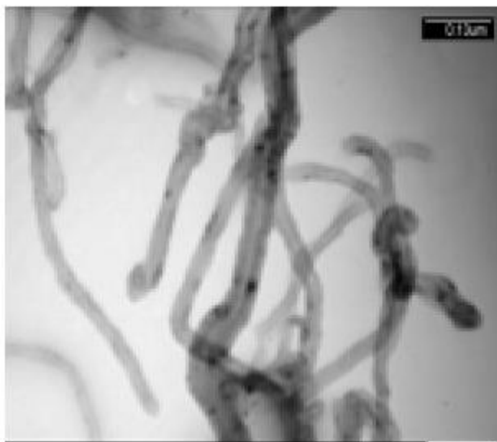
Fig.1 TEM image of purified MWNTs
